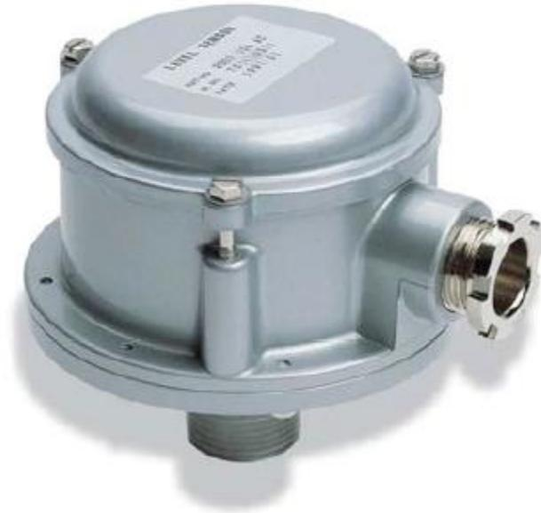
The Series NLS pneumatic liquid level switch is designed for use in high viscosity liquids. It is modified to overcome the high viscosity by making the tip of the detecting pipe larger than usual. The NLS is the ideal sensor for applications where electrical power is not available or hazardous conditions exist. Using a diaphragm, the switch is actuated by compression of a captive air column in the detecting pipe beneath the diaphragm.
